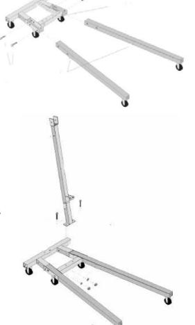
**Step 2,** Using bolts two bolts #12 washers #? and nuts #2 securely fasten post #10 to base.
