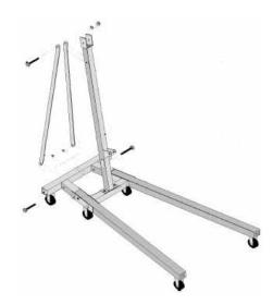
**Step 4,** Position boom #13 into the top of the post, using bolt #14 washer #? and nut #? fasten in place
