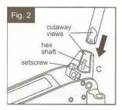
At the rear of jack a large wire retaining clip holds handle base (Fig.2, part C) flat against the jack.
